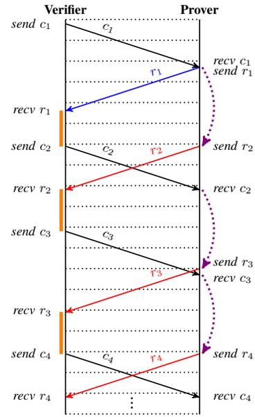
Fig. 5. A challenge-response sequence involving a guessing-ahead prover. The dashed horizontal lines mark the verifier's discrete clock cycle boundaries, and the vertical bars on the left highlight the verifier's (variable) processing delay.
